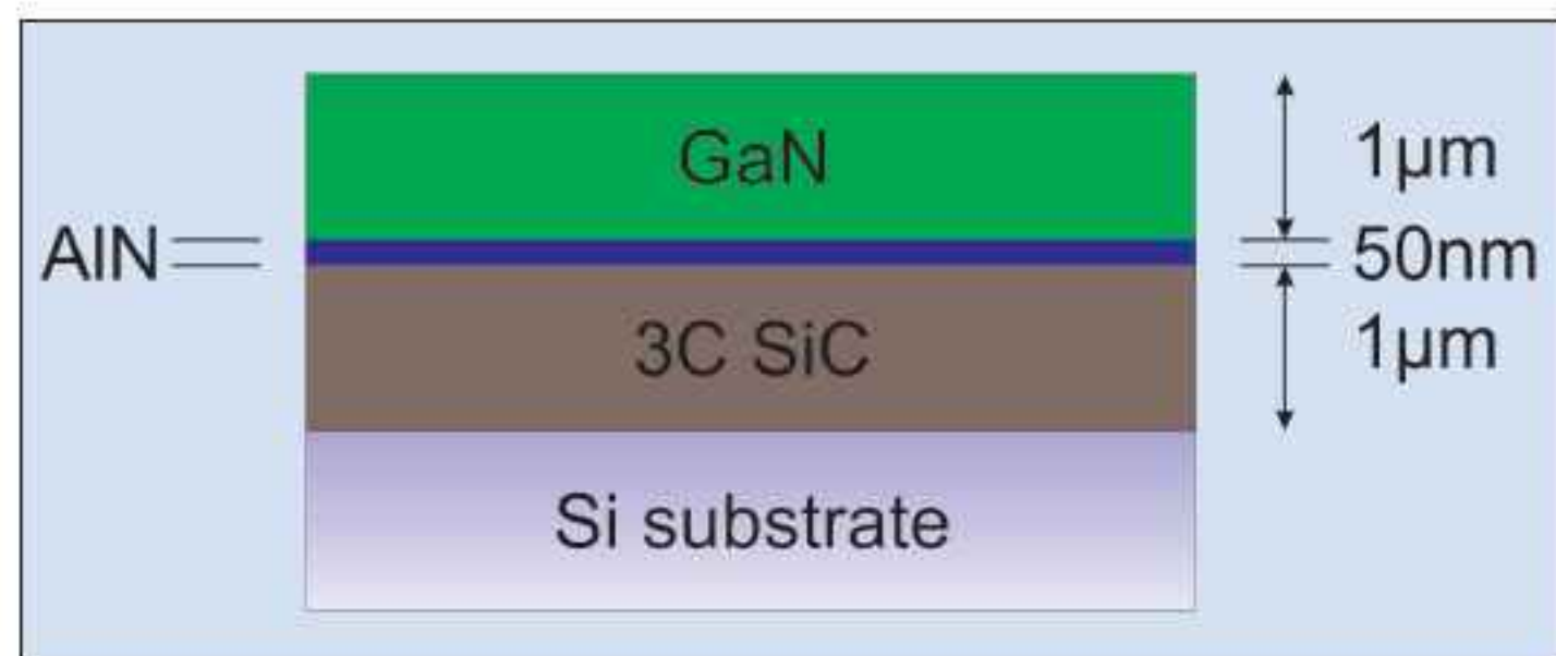
Figure 2. Covalent's GaN/SiC/Si layer structure with AlN buffer. The SiC crystal structure is oriented [111] and the xN [0001].
